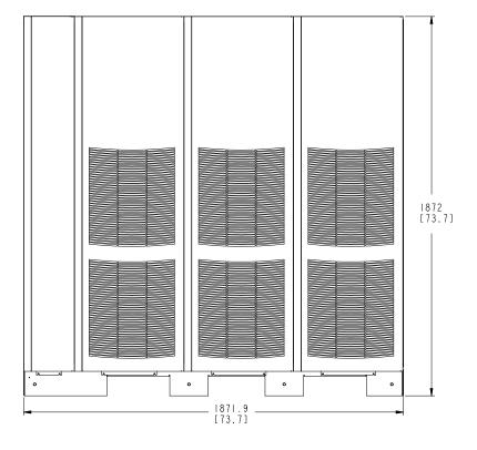
Figure 3-4. UPM Section Dimensions (Front View)
